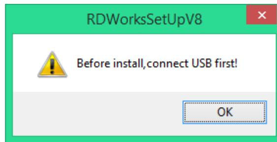
The setup program will ask you to connect the USB cable from the computer to the laser machine (and turn on the laser machine). Click the [ OK ] button.
