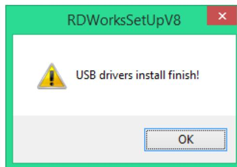
After the USB drivers have been installed, the setup program gives a message that the "USB drivers install finish!". Click the [ OK ] button.
